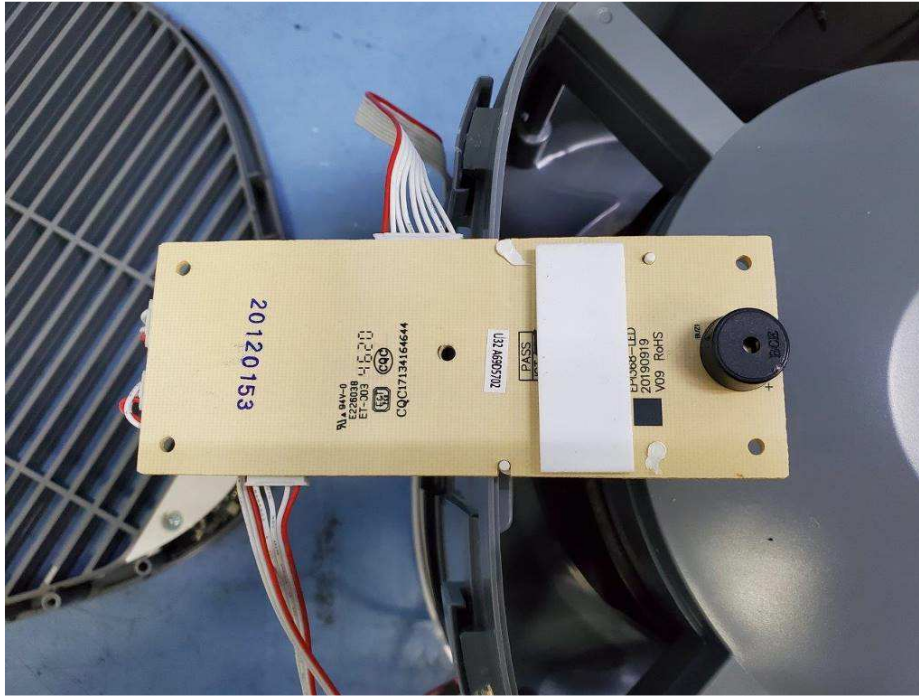
Display PCB back view
