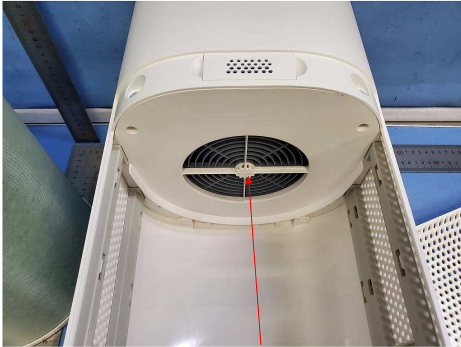
Air inlet, UV lamp position
