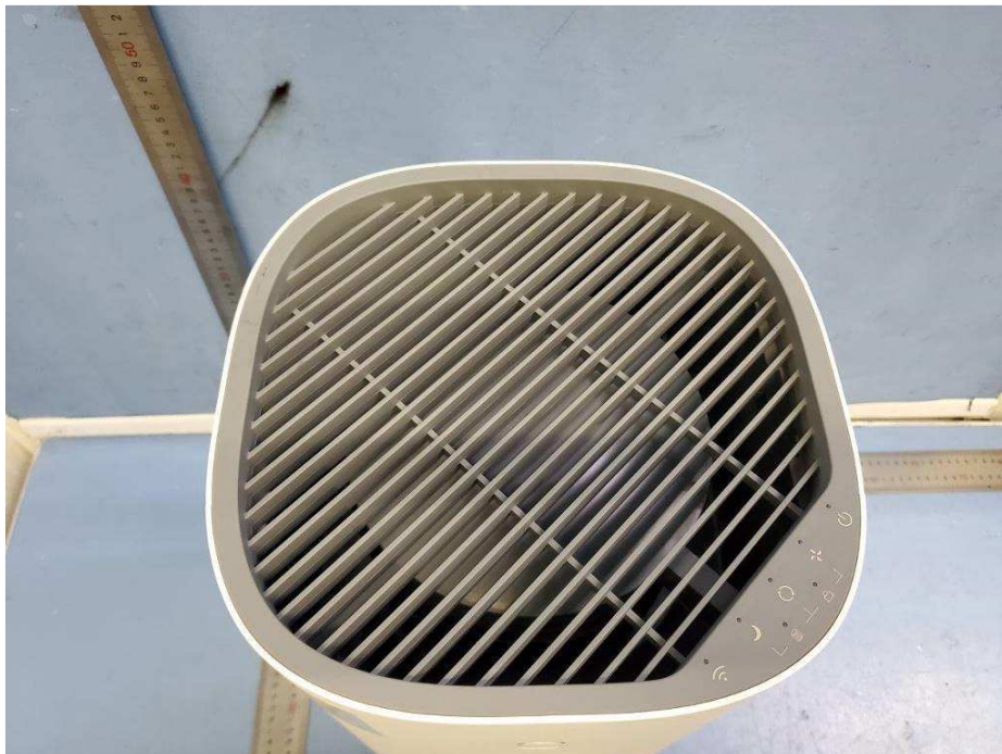
Top view (Air outlet and control panel)
