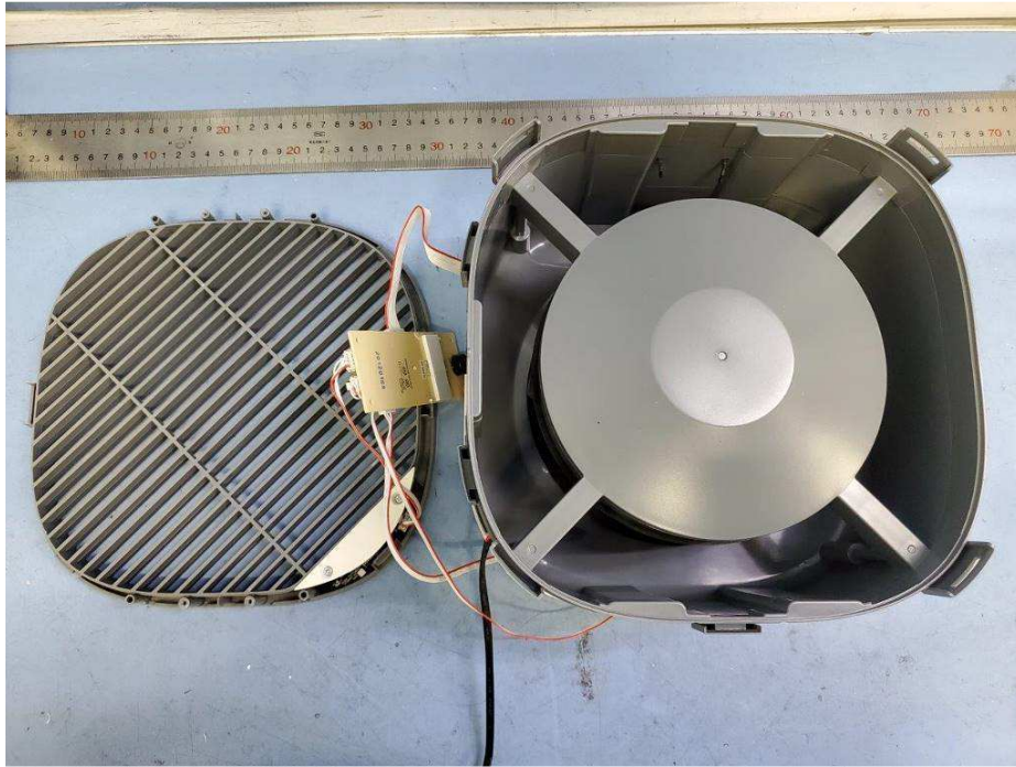
Remove air outlet grill view
