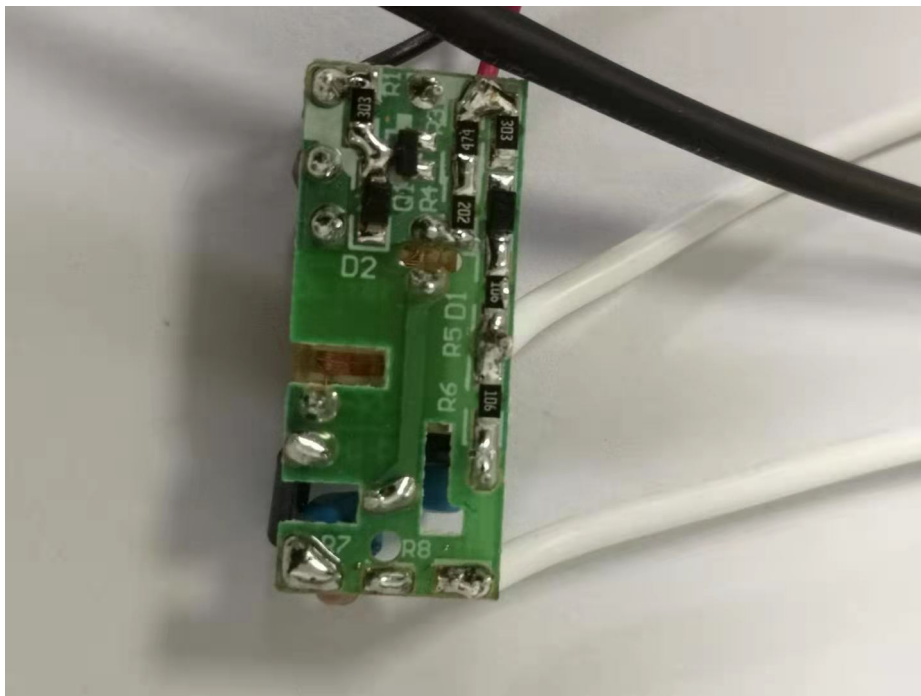
Bottom view of Anion generator
