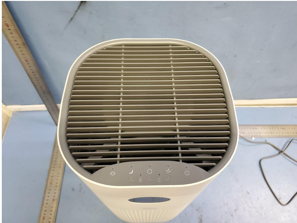
Air outlet and control panel
