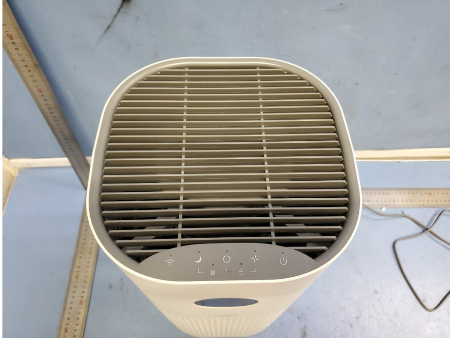
Air outlet and control panel
