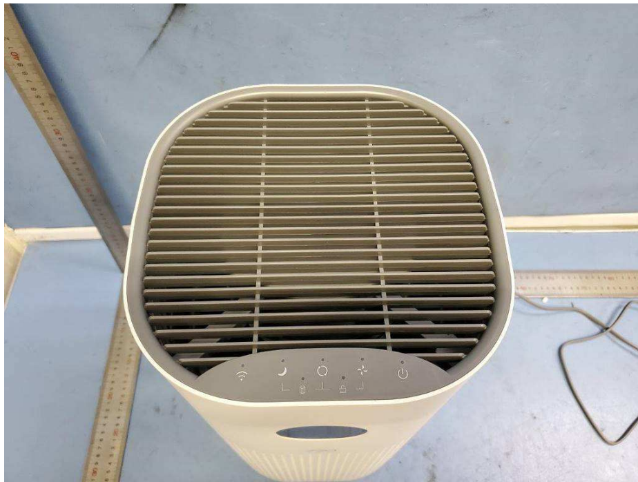
Air outlet and control panel
