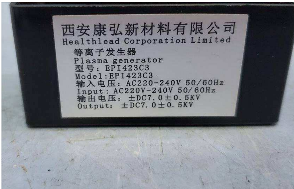
Plasma generator for model DS-S800, DS-X1000N-A and DS-X1000W
